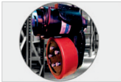
Upper horizontal driving wheel
