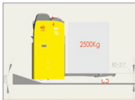
1. With strong power and good throughput capacity, gradeability under unladen can reach 25% and arrive 10% under laden situation. 2. Lift height of 135mm is better for pallets applicability.
