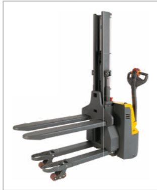
With double decker ,mast lift 1000kgs and support arm lift 1000kgs, total load is 1000kgs if using double pallet.
