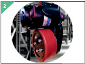
Upper horizontal drive motor to make replace driving wheel easier
