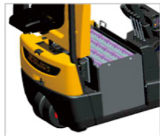
Sideway battery box
