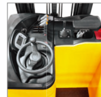
Large cab with dead man power off switch, Multi-function display: battery state, hour meter, fault indicator etc.
