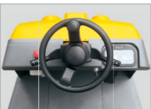
Adjustable steering column with electric F/R lever.
